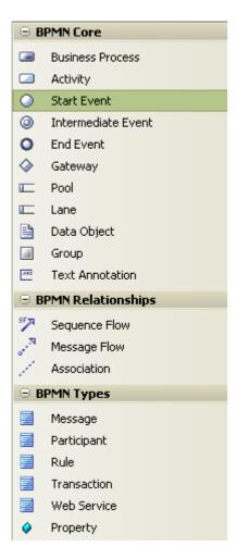
The BPMN Toolbox pages provide the graphical (Core) and non-graphical (Types) Business Process Modeling Notation (BPMN) elements for use on business process diagrams. Specifications of these elements and relationships are defined by Tagged Values.
